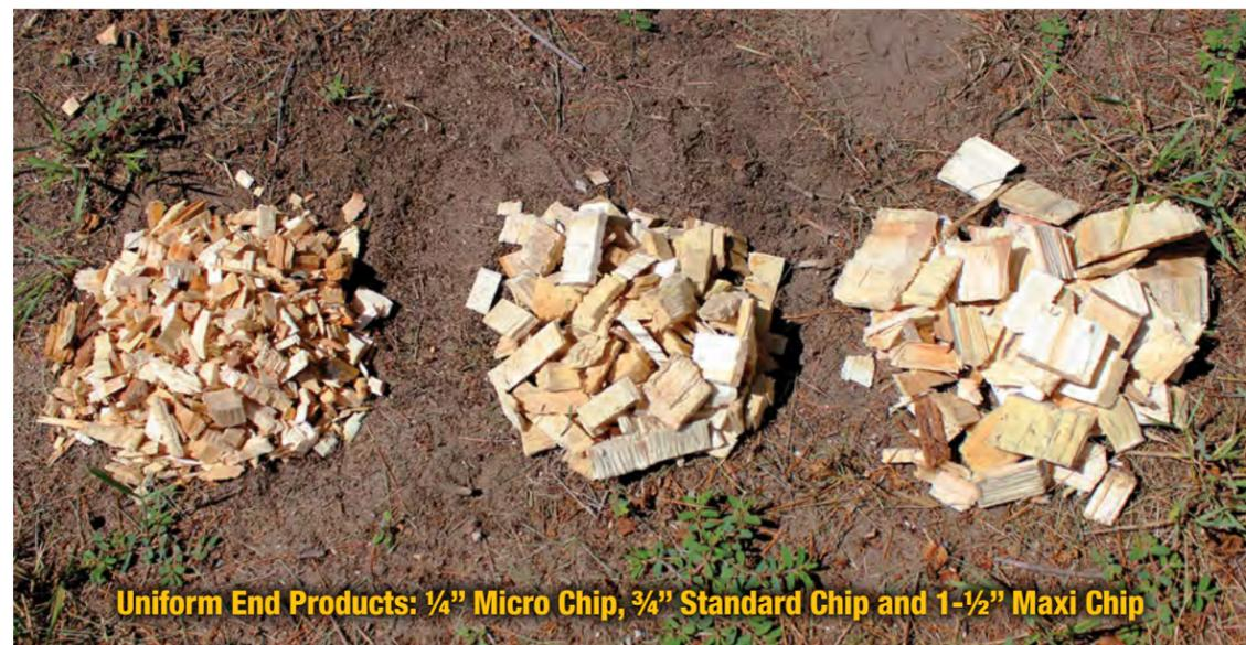
**Uniform End Products: 1/4" Micro Chip, 3/4" Standard Chip and 1-1/2" Maxi Chip**
