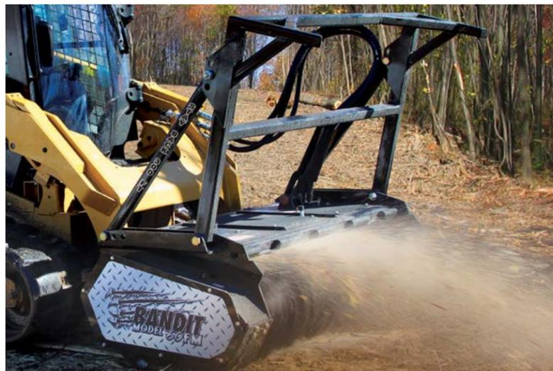
The strength of Bandit's forestry mulching attachments is their ease of use. They attach quickly via a quick attach plate and are operated by the loader's existing hydraulic systems. That means it takes only a few moments to attach either the Model 60FM or the Model 72FM and get to work. The loader powers a single variable speed hydraulic motor on the mulching head, giving the mulchers impressive grinding power with very simple maintenance.
